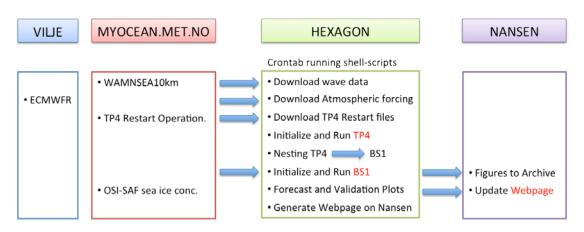
Figure 2. Schematics of computer resorces used for the forecast system
